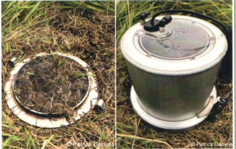
Dual head infiltrimeters record the ease with which water infiltrates the soil and provide a vertical flow rate metric.
