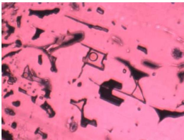
**Figure 1.** Infrared light photomicrograph of two-phase fluid inclusions within Buckskin-Rawhide hematite.
